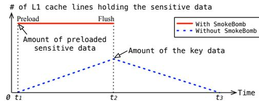
**Figure 1: The difference in cache usage with and without SMOKEBOMB.** The  $x$ -axis denotes the time of code execution and the  $y$ -axis represents the number of cache lines holding sensitive data. Any observable changes on the  $y$  access represent a potential cache side-channel attack vector.
